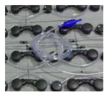
The electrolyte circulation system ensures a permanent electrolyte movement inside the cell. The air pumped into the base of the cell maintains an electrolyte circulation offering lower water consumption, lower battery temperature and long life.
